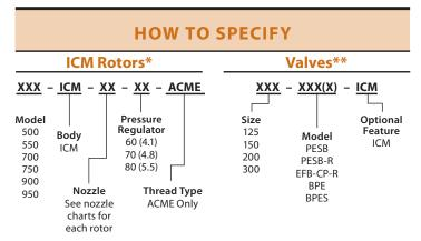
\* For exact combinations of Rotors (Nozzles and Pressure Regulator) see pages 33–41 for correct model.
