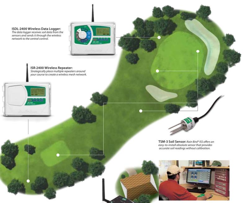
**ISG-2400 Gateway:** Located at the computer, the gateway is the link between data loggers and repeaters in the field and the Soil Manager™ software.
